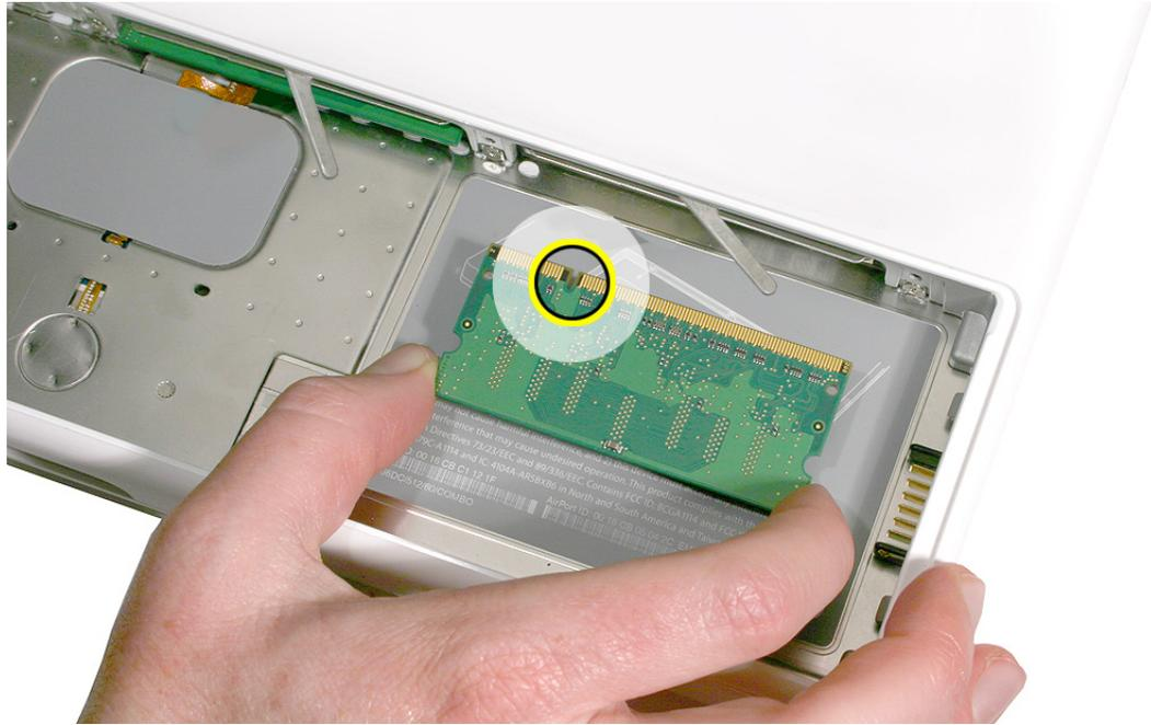
2. Use two fingers to push firmly on the edge of the memory cards. If there is a tight fit, installing the cards may take some force to ensure that they are fully inserted.
