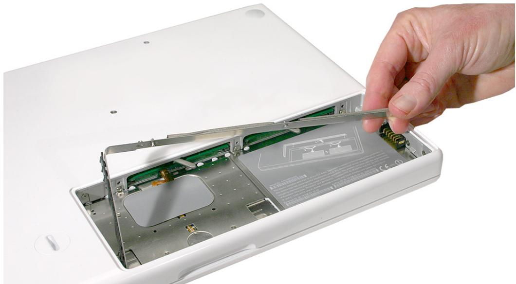
3. **Important: Remember to replace the RAM door after you have finished working inside your computer. The computer will not function properly if the RAM door is not replaced.**
